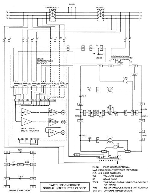
Consider the Robonic II in the normal operating position, with normal power available and the normal interrupter closed. The following are energized: U.V. (undervoltage module), TDES (time delay engine start), and NR (normal relay).
